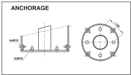
Base -038-Bolt M<sub>10</sub> Nut M16 Washer Flange F100A
